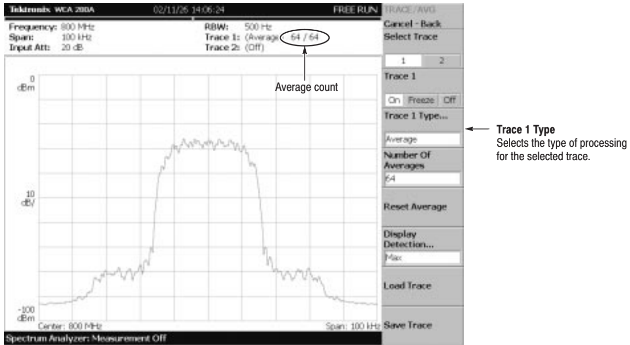
Figure 2–23: Comparing a new waveform with an averaged waveform
