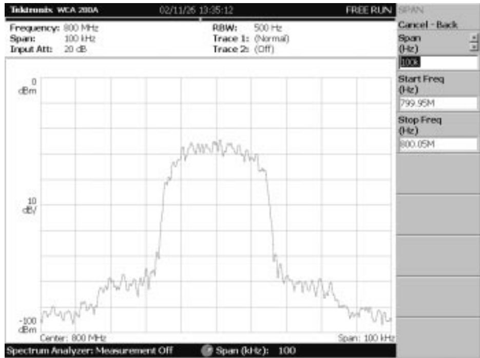
Figure 2-15: Center frequency of 800 MHz, span of 100 kHz
